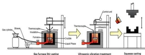
Fig. 1. Combined rheo stir squeeze casting process.
