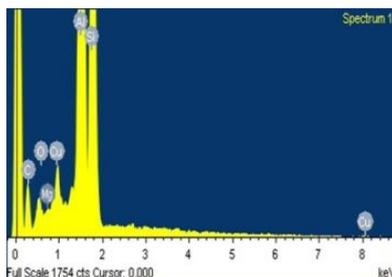
Fig. 4. (a) Metallurgical micrograph of RSC AlSi17 alloy, (b) Metallurgical micrograph of CRSS casted AlSi17 alloy and (c) EDS analysis of AlSi17 alloy
